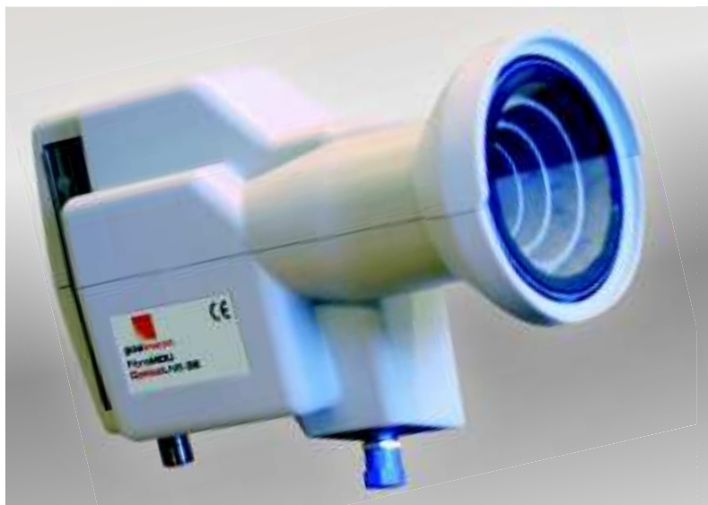
(below) The Fibre Optic LNB can feed the whole Ku-band to up to 32 end-points. That F-connector is just for power
