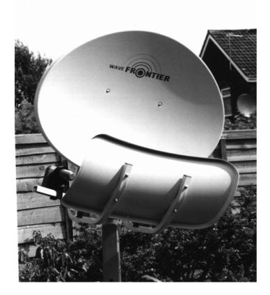
Note the amount of tilt on the dish, this is to account for the elevation angles between satellites  $55\ \mathrm{cm}$
